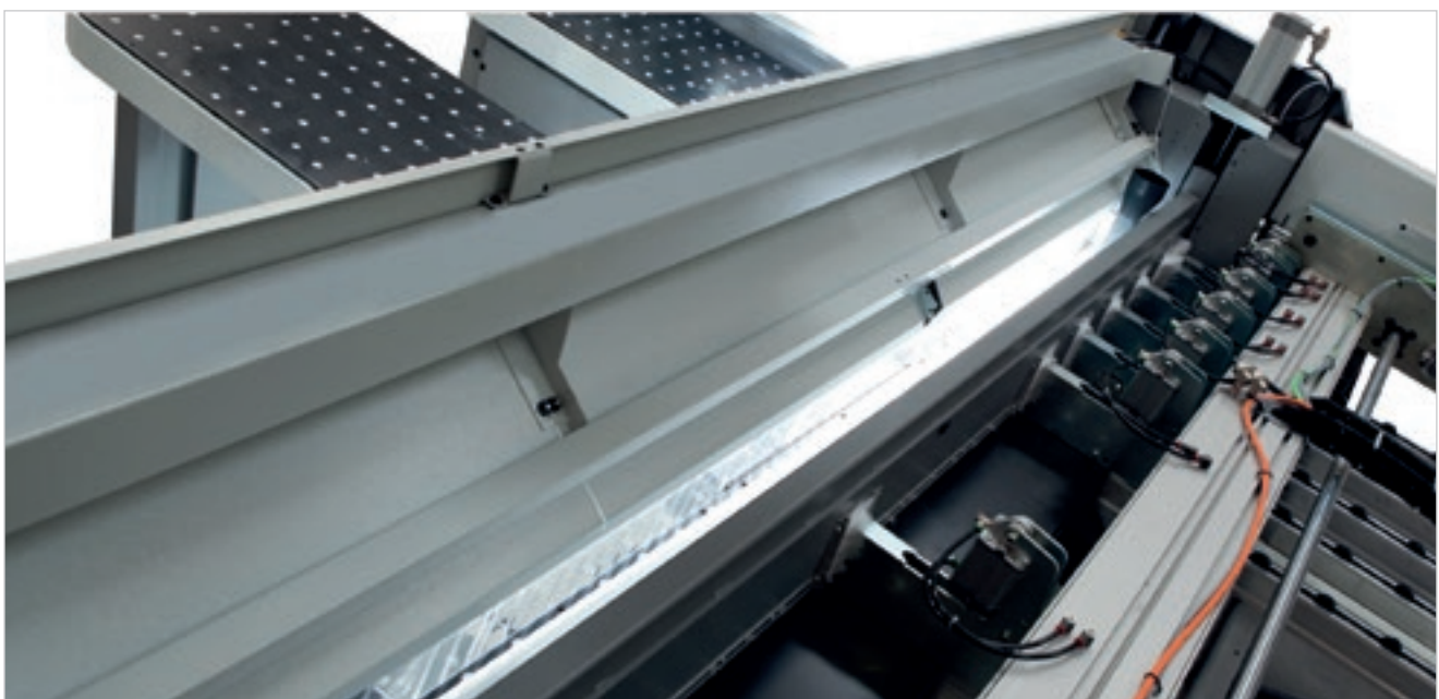
The pressure beam has a single structure for an even pressure on the stack of panels to be cut. The opening is automatically adjusted by the numerical control in relation to the thickness of the stack to be cut, thus obtaining the best cutting quality under any working condition. (Not available on Sektor 350).
