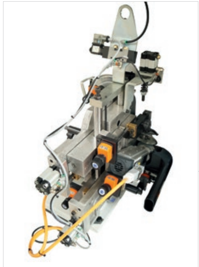
The Fine trimming unit trims the top and bottom of the edges with 2 high-frequency motors and vertical / horizontal rotating disc copiers.
